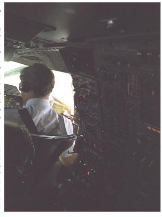
engine number 3. As we were flying at above 250 knots, the visor and nose were both in the 'up' position, restricting the view out of the window. The number one autopilot was engaged holding the airspeed constant as we descended at fixed power. The autopilot control panel is visible just below the central spar in the middle of the window.
