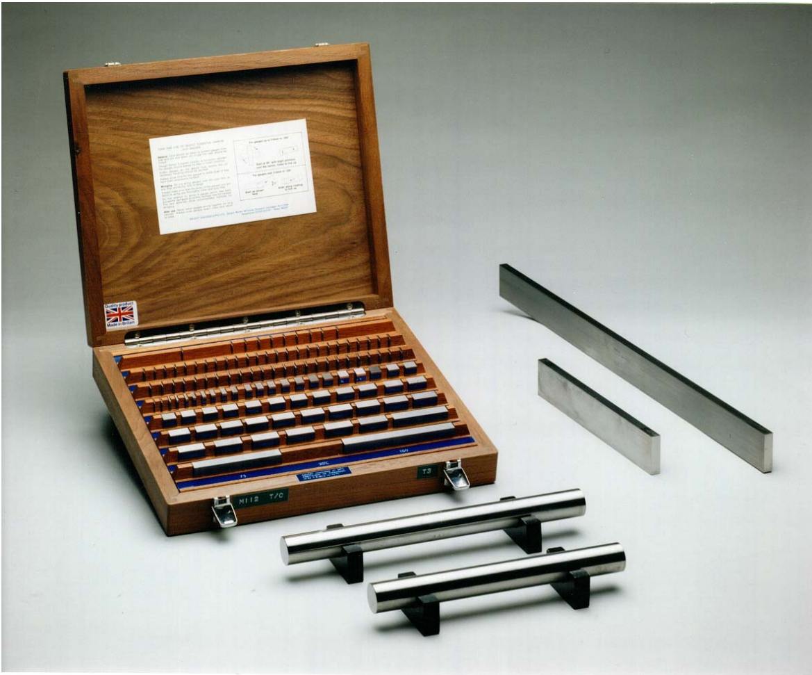
Figure 1.4 - A set of gauge blocks, 2 long series gauge blocks and 2 length bars (foreground)
