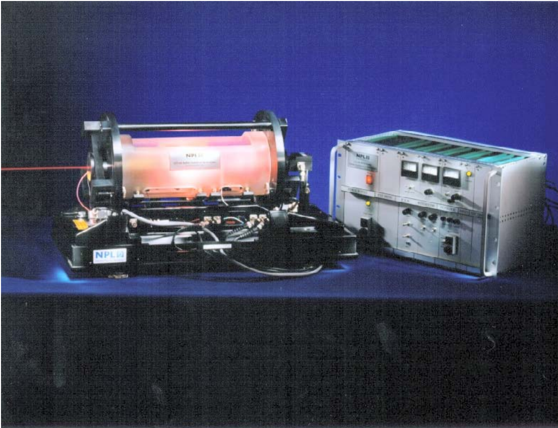
Figure 1.8 - Iodine-stabilised He-Ne Primary laser
